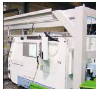
Lathe with digital control
