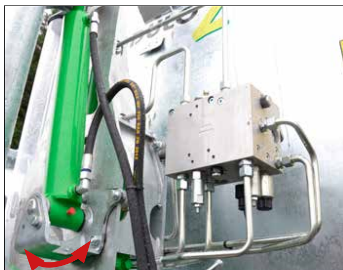
To switch sides, the base of the hydraulic ram only has to be moved from right to left
