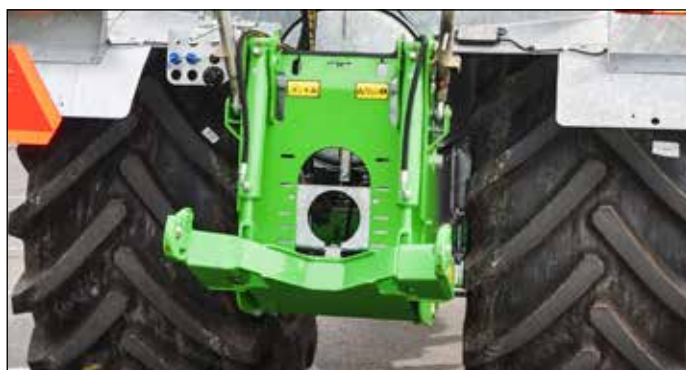
L600 linkage on COBRA (fastened by 4 tapered shafts to make it a solid construction)
