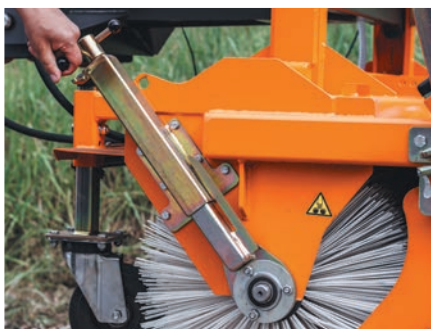
Stepless spindle adjustment of the main brush
