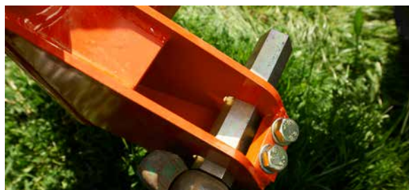
The linkage pins are easily adjusted to match the tractor width, which enables the mower to cut to its' full working width.
