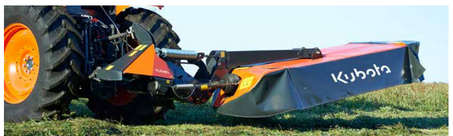
Lifting on headlands via hydraulic cylinder – ample ground clearance.
