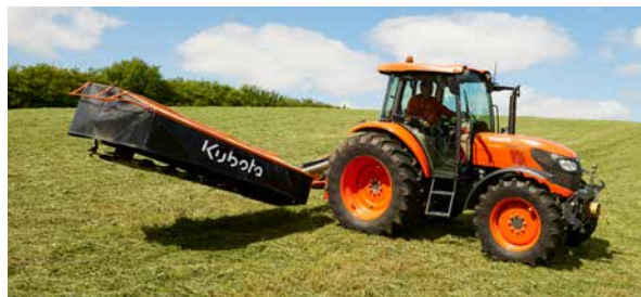
Lift on headlands via a hydraulic cylinder – no use of the 3-pt hitch is needed.
