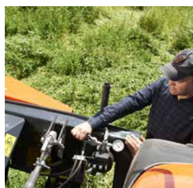
Hydraulic setting of ground pressure.
