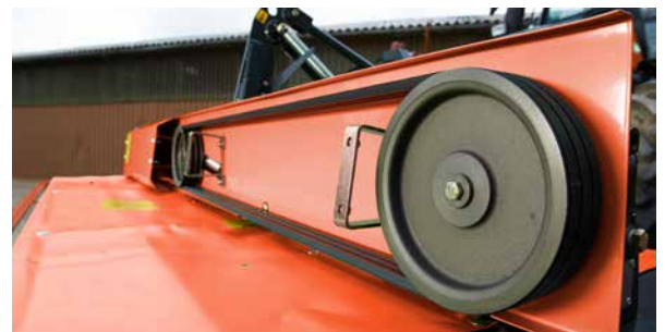
By switching driveline pulleys changing from standard PTO speed of 1000 rpm to 750 rpm is possible.
