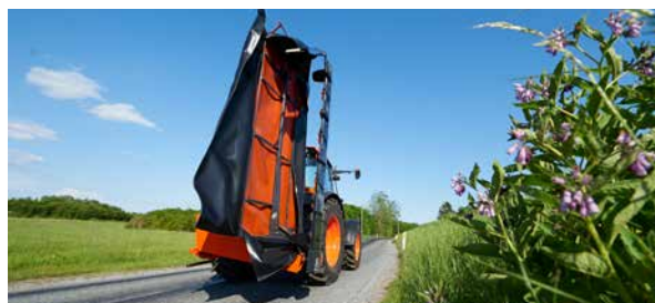
For transport the machine is folded hydraulically from the tractor cab to the vertical transport position well behind the tractor, ensuring a stable and steady transport.
