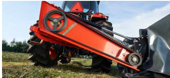
Four v-belts ensure excellent transfer of power.
