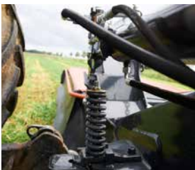
When encountering an obstacle the NonStop Break-Away system protects the cutterbar by swinging it back and up.
