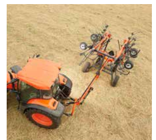
80° turning angle ensures excellent manoeuvrability.
