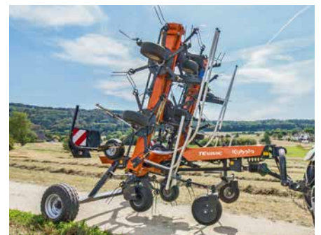
Standard running wheels of both models are extra wide 10.0/75 – 15.3 tyres with a generous track width of 2.45m.
