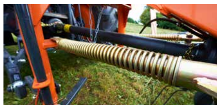
Standard oscillation dampers on TE6060 ensure an even spreading pattern.
