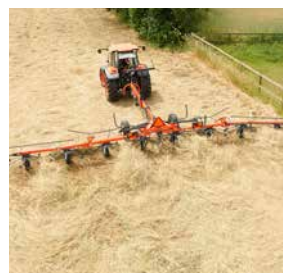
For border tending the outer rotors are pivoted, to secure evenly inward spreading.
