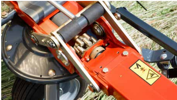
HexaLink finger clutch permits the rotors to fold 180° for transport.
