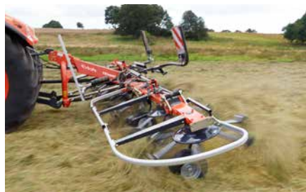
New aluminium rail guards, which are low in weight, but still extremely impact resistant.
