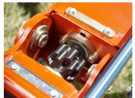
Kubota HexaLink finger clutch permits a 180° folding of the rotors for transport.
