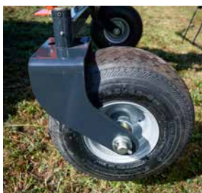
New optional third wheel with tandem axle for high accuracy in ground followings.
