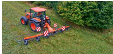
Central adjustment for border tending is standard on all models.
