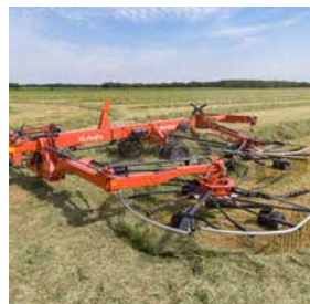
The two outer rotors can be adjusted individually to match a working width between 9.50-15.00m.
