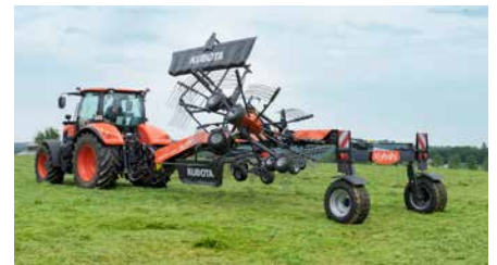
Ground clearance >500mm.
