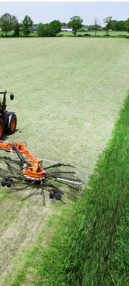
The two outer rotors can be adjusted individually to match a working width between 9.50-15.00m.
