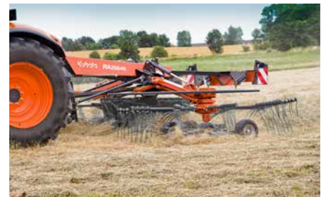
Better ground adaptation compare to larger single rotor rakes.
