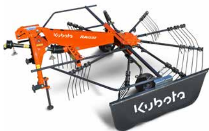
RA1032 – compact entry-level 3.20m rake with a weight of only 320kg.
