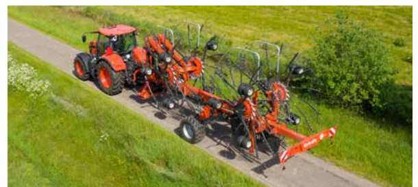
With its clever folding mechanism the total height remains below 4.00m - despite a rotor diameter of 3.85m. And there is no need to remove tine arms for road transport.
