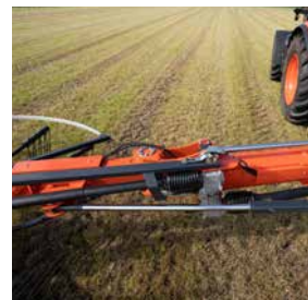
Hydraulic suspension of front lift arm and Break-Back system.
