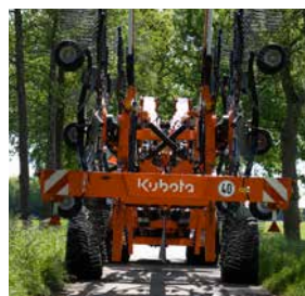
With its clever folding mechanism the total height remains below 4.00m - despite a rotor diameter of 3.85m. And there is no need to remove tine arms for road transport.
