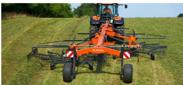
The side delivery concept allows you to collect crop from 15.00m into a single swath.
