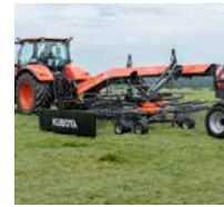
Automatic fold-able swath board with parking stand.
