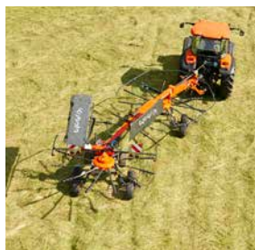
SideShift to the left - raking without driving on unraked crop.
