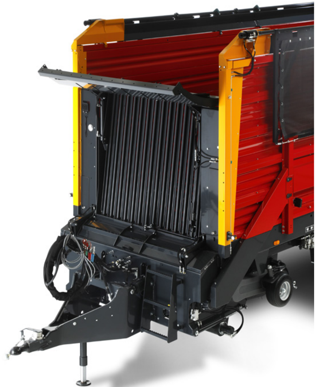
Rapid Stream front panel in maize silage harvesting position
