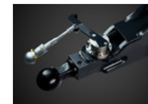
Electric steering. Standard on 7200 and 8400+ models. Optional on other models.
