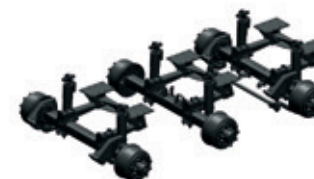
40 tons hydraulic suspended forced steered tridem
