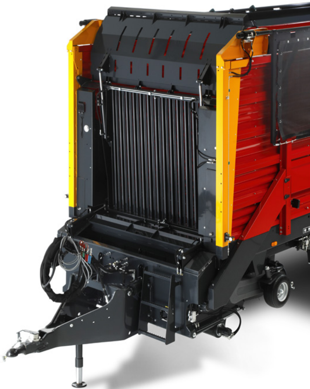
Rapid Release front panel in unloading position
