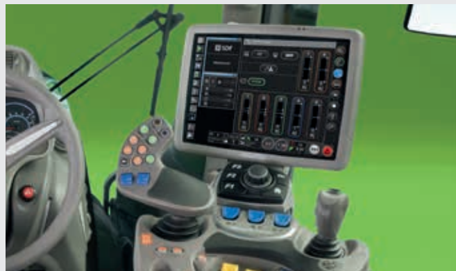
↑ Electric spool valves with comfortable electronic control elements.
