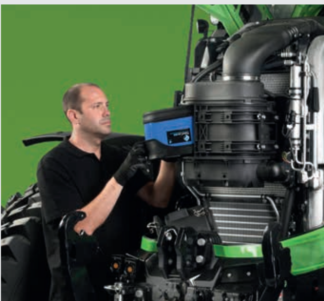
↑ Easy access to the PowerCore air filter.
