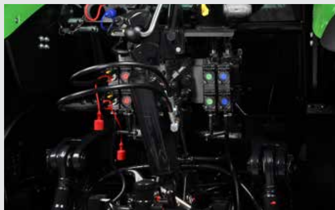
↑ High comfort combined with ease of use: mixed hydraulic configuration with two electric and two mechanical distributors.
