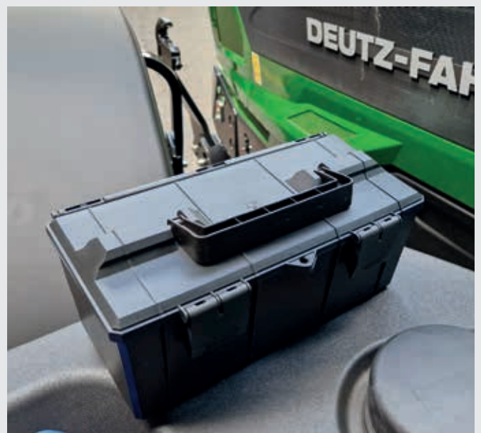
↑ Storage box above the fuel tank on left side for air hose and air gun.
