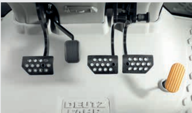
↑ Ergonomic engine brake activation via foot pedal.
