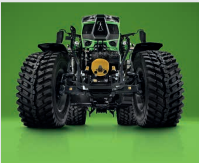
Front linkage with up to 5450 kg lifting capacity and optional DualSpeed front PTO.
