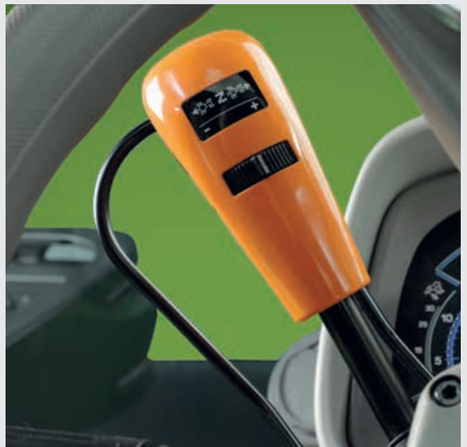
↑ Ergonomic PowerShuttle lever with SenseClutch adjustment dial.
