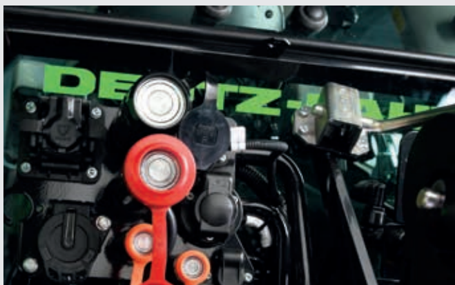
↑ PowerBeyond available with standard or flat face couplers.
