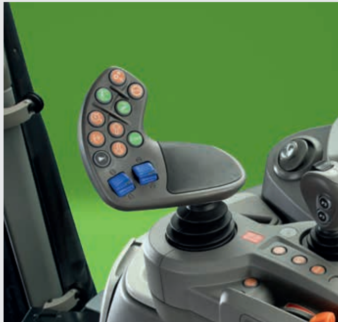
Simple and intuitive transmission management through the practical and ergonomic MaxCom joystick.
