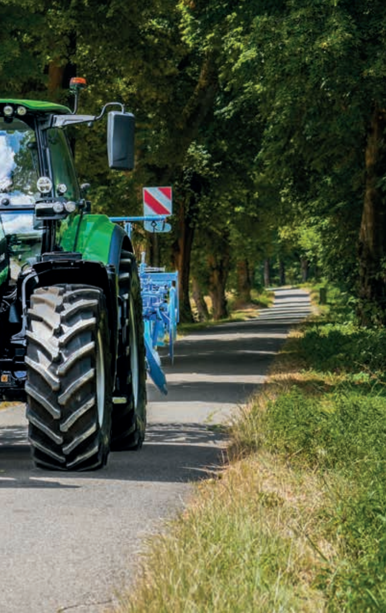
↑ The new front axles offer higher axle loads and integrate a new suspension sensor.
