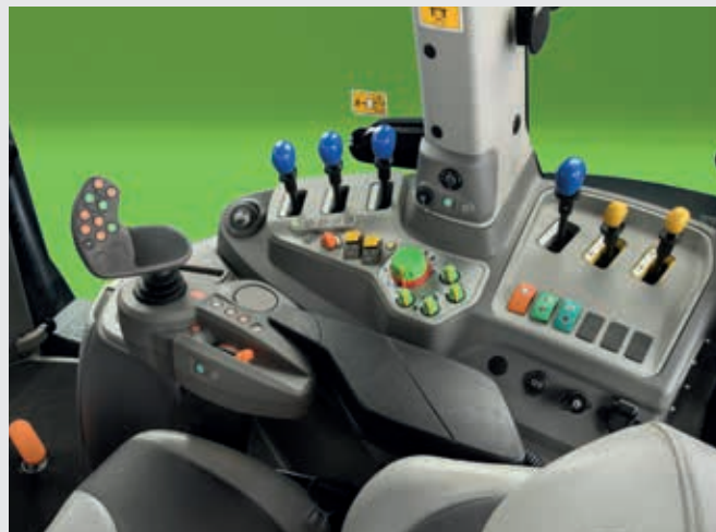
MaxiVision cab equipment with full mechanical rear spool valves is available for Powershift (large picture) and RCshift (picture above) models.
